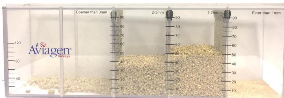
7. Record the values for each compartment using the left scale of each compartment.
